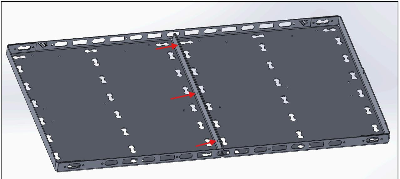
Next slide the two connector braces into the slots on the front and back of the platforms and bolt through the outside face using **(4) M6x14mm Button Head Bolts** and **(4) M6 Lock Nuts per side**
