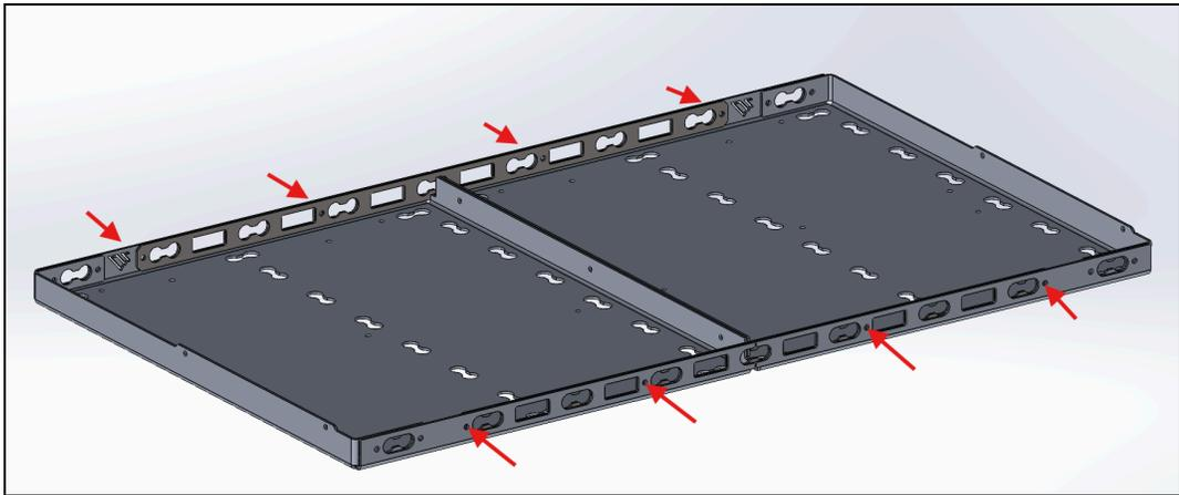
Next we will attach the left and right edge guards through the top of the platform using (2) **M6x14mm Button Head Bolts** and (2) **M6 Lock Nuts** per gaurd.
