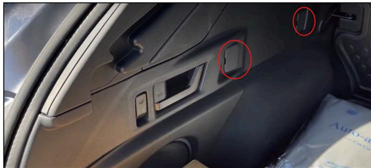
Pop open the cover using a thin screwdriver. Do this on both sides (4 total).
