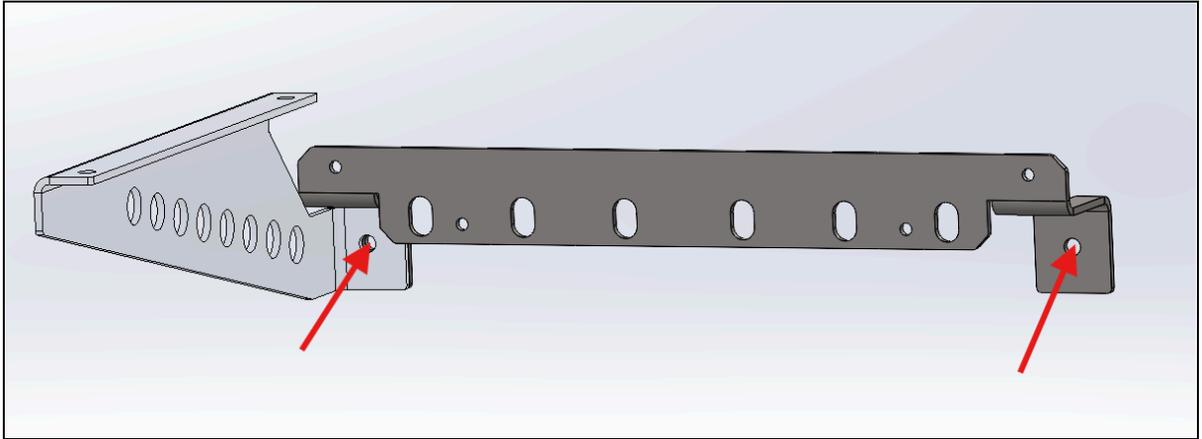
Next attach the molle panel using **(2) M6x14mm Button Head Bolts** and **(2) M6 Lock Nuts** per side
