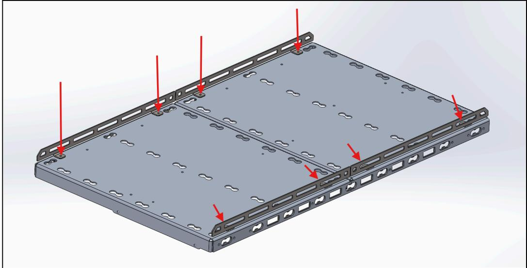
Now set the platform on top of the mounting pieces and bolt into place using (2) **M6x14mm Button Head Bolts** and (2) **M6 Lock Nuts** per side.
